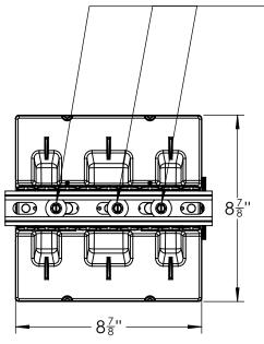
Proper installation of strut requires 3 #14 X 1" hex screws with 1/4" washers (hardware included with ROL-06).
